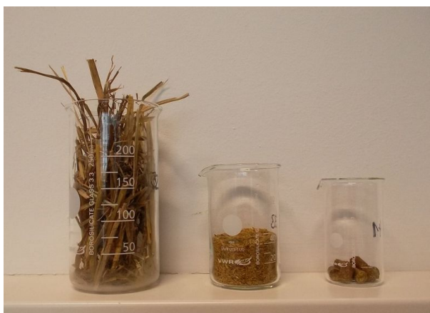
Comparison of straw sample volumes with the same mass (input material, after hammer milling, pelletised)
