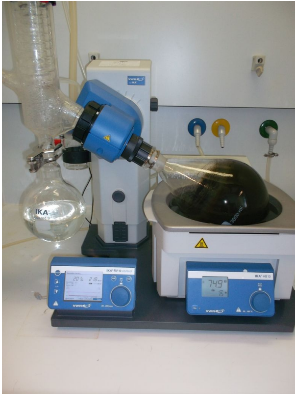
Laboratory reactor for evaporating digestates
