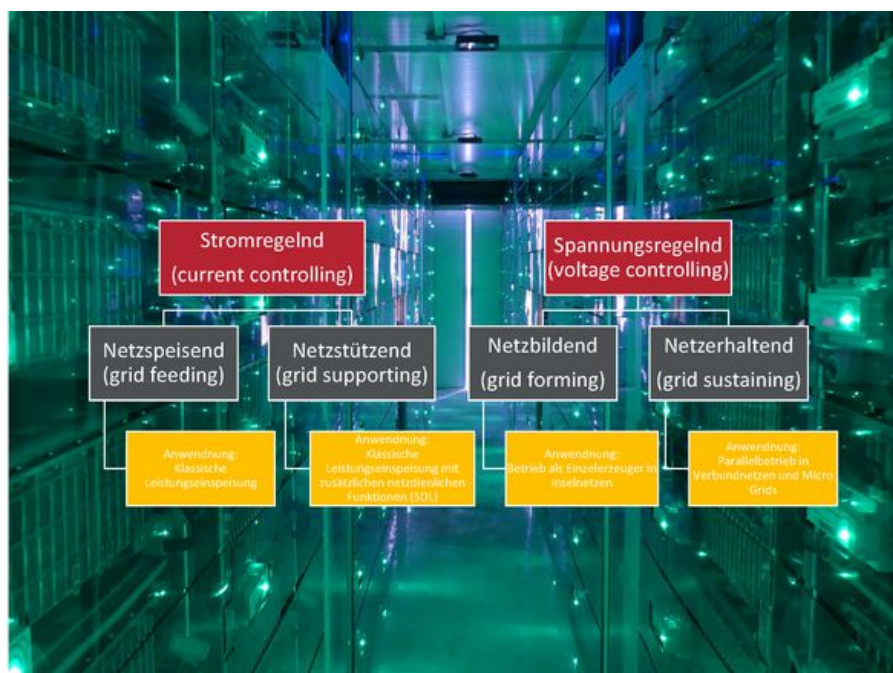
Possibilities for providing control and grid stabilisation by using inverters
