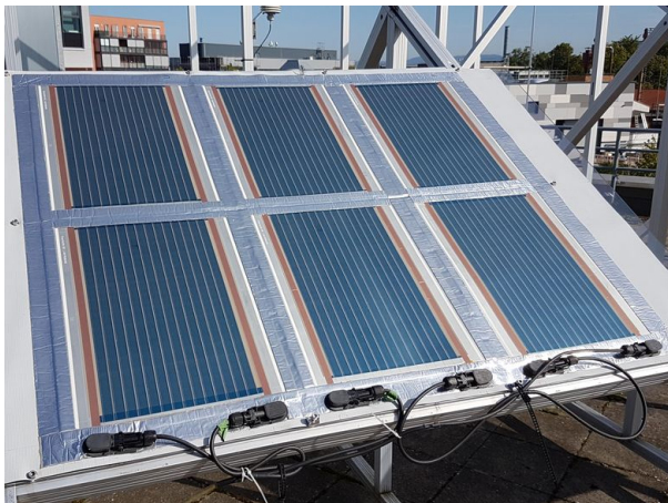
Organic solar cells without indium tin oxide (ITO) on a flexible foil.
