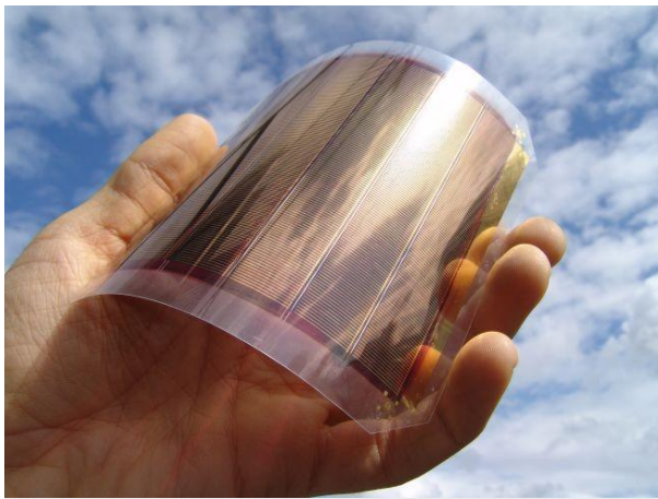
Organic solar cells without indium tin oxide (ITO) on a flexible foil.
