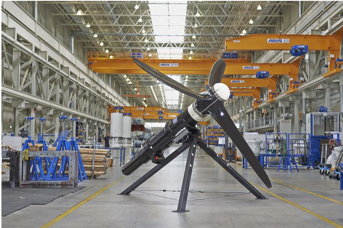
SIT 250 turbine in production at SCHOTTEL in Dörth, Germany
