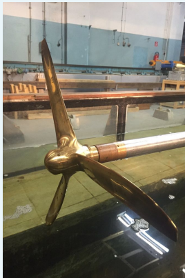
Turbine model rotor in the tow tank at SVA Potsdam
