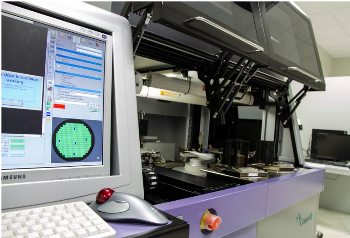
A wafer for concentrated photovoltaics in an automated optical inspection (AOI)
