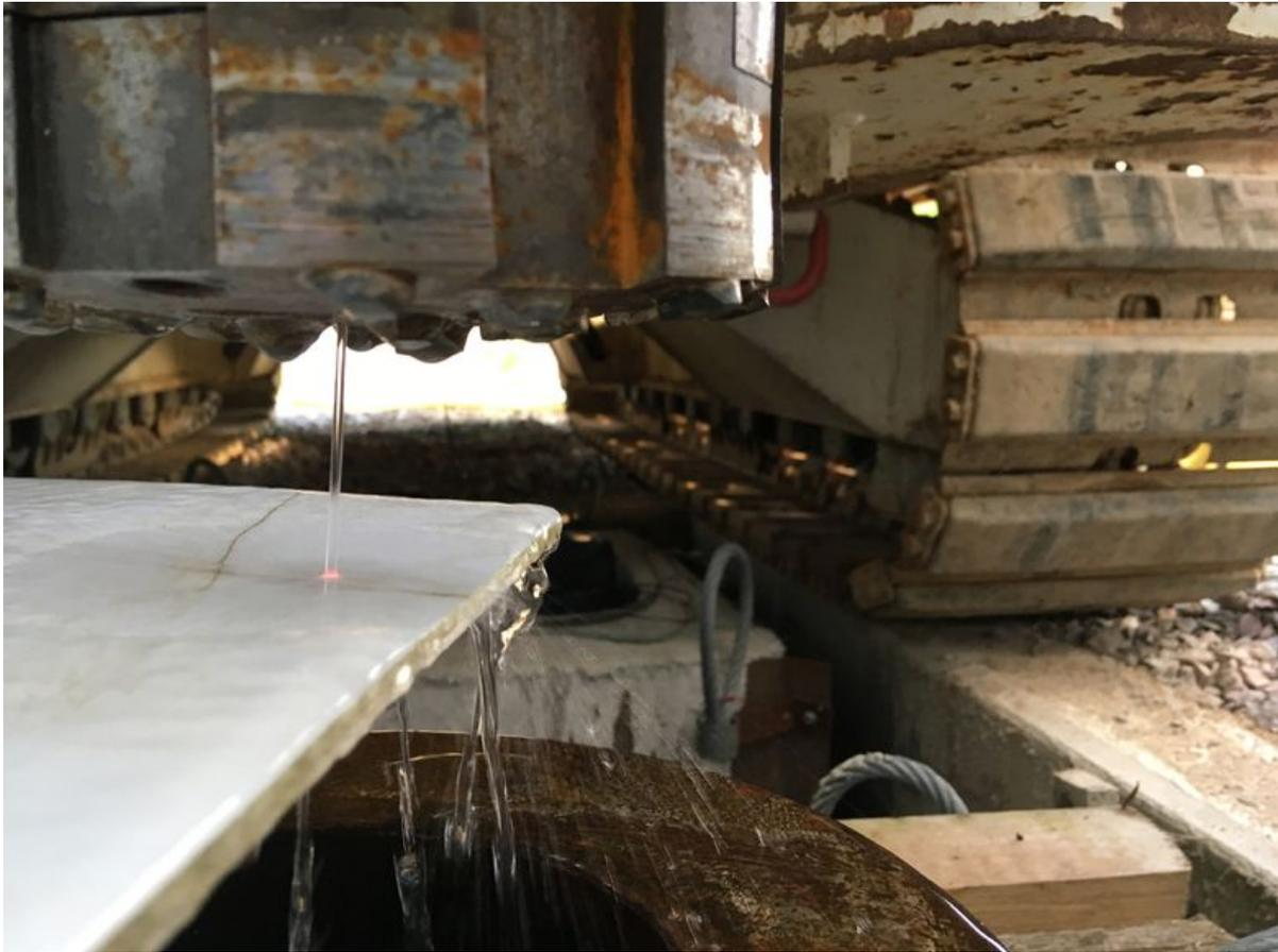
The drill head with integrated laser head is located at the end of the hybrid drill string. The emerging laser-water jet is clearly visible.
